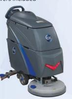
i20NBT, 20" Traction-Drive 15-gallon solution tank; 66 or 99 lbs pad pressure; 30" squeegee; on-board charger; 19" pad driver included
